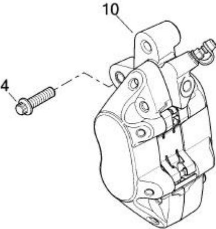
Mount the new TB brake caliper adapter to the front fork using the included screws. Tighten the screws with 35 Nm (25 ft-lbs) torque.
