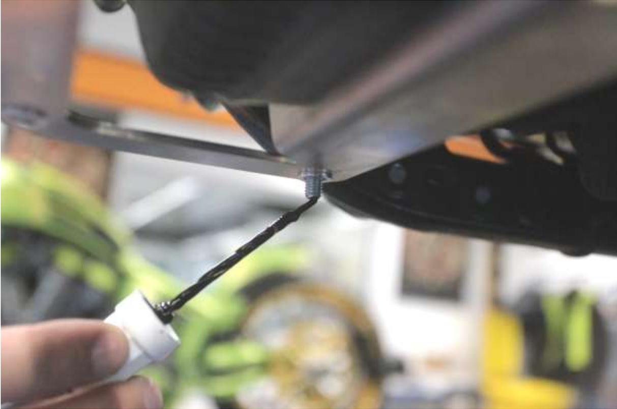
Push the chin fairing to the bracket from underneath so the marked screws will mark your drilling holes into the chin fairing.
