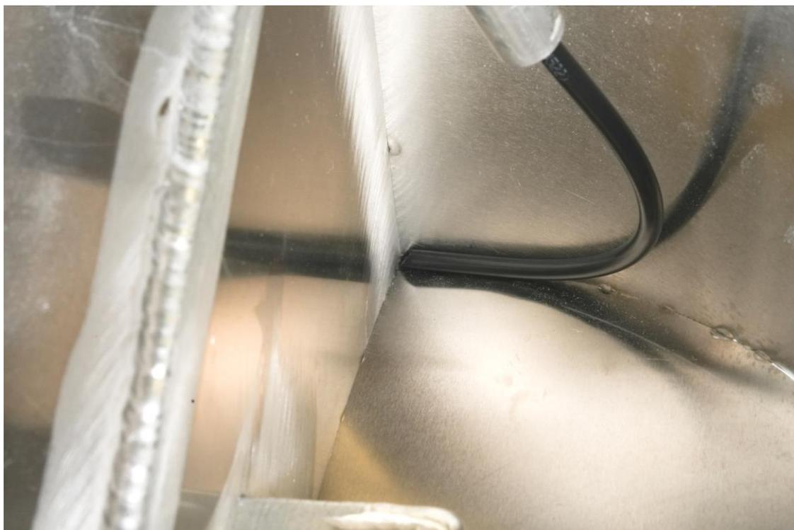
Picture shows diagonally cutted hose inside of the fuel tank
