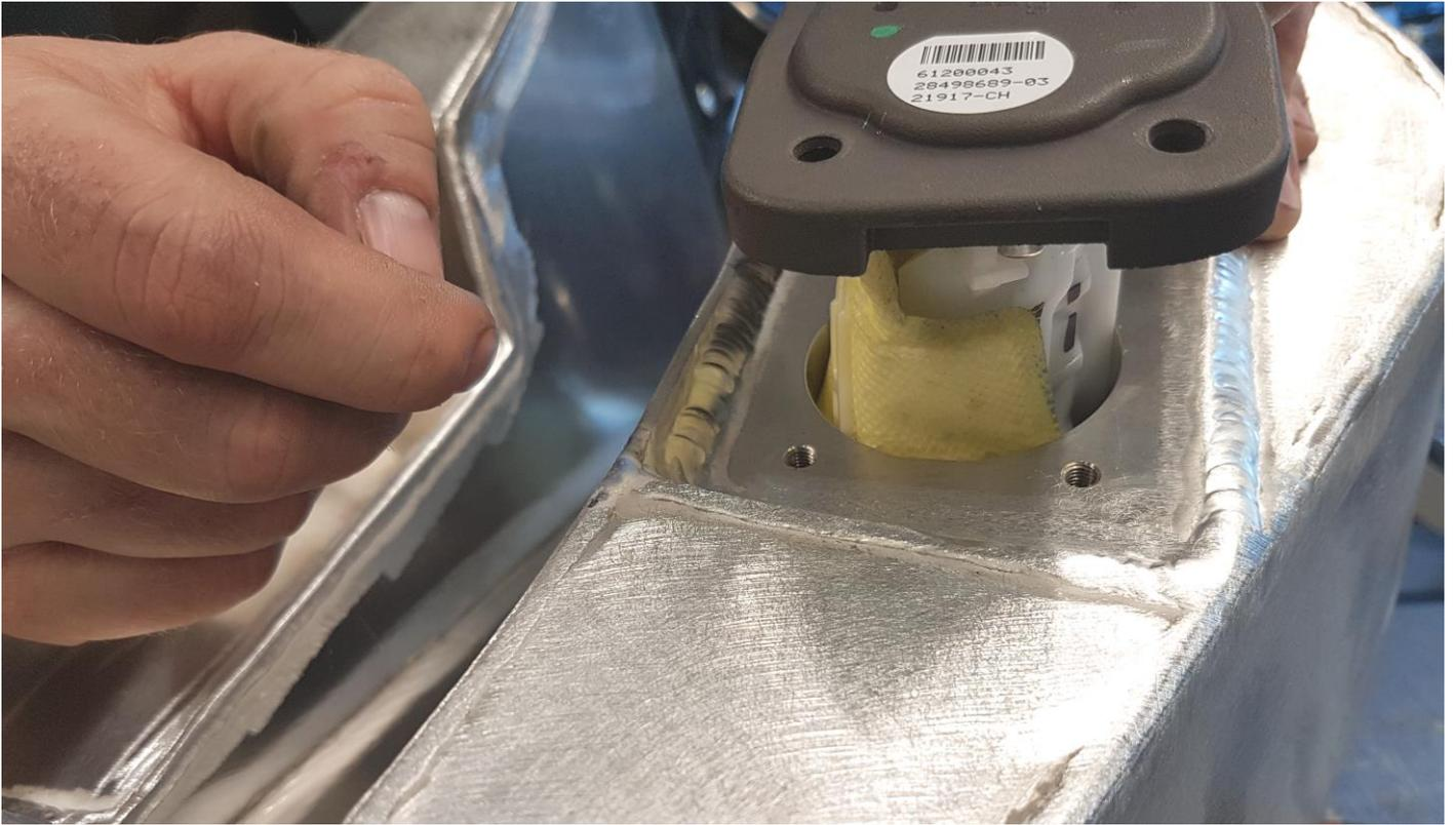
Mount the ground plate using the included M5 screws with washers.
