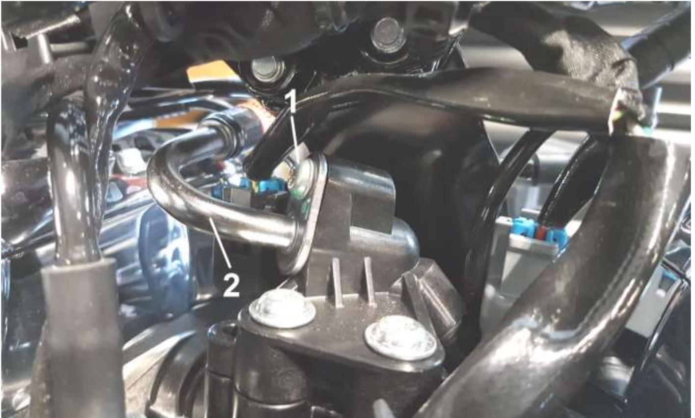
Open the sheet on fuel hose end by a rasp and push off the hose.
