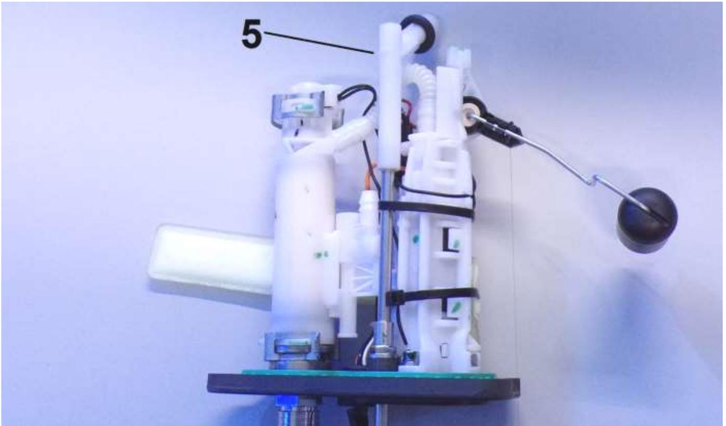
Push the fuel pump into the new tank, first part inside has to be the floater. Take care the yellow filter unfolds inside the tank.
