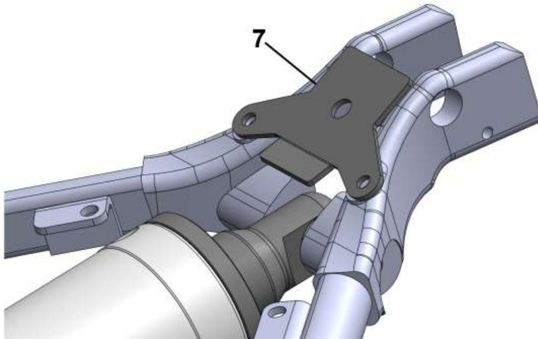
Mount the front of the tank with the included mounting kit and the plastic washers.
