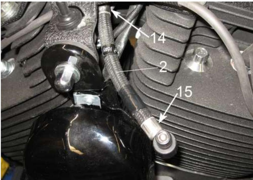
Cut off the sockets (14 + 15) of the fuel line carefully. Replace the OEM fuel line (2) by the new part. Place fuel line to the fuel pump; make sure it doesn't scratch on parts of frame or engine and the line is not under tension!
