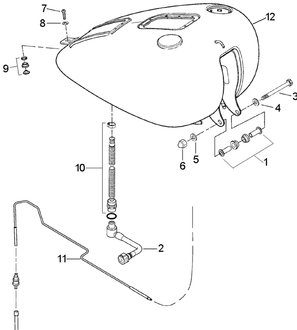
Parts (1) and (2) will be used again; the other parts in picture above will be replaced by new parts.
