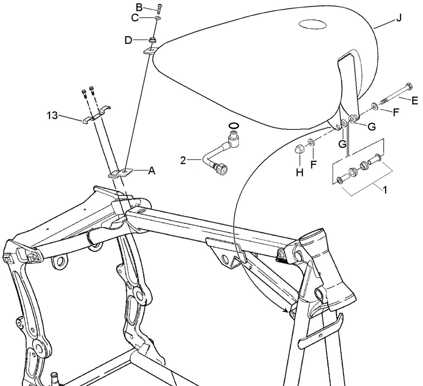
Install the tank with the parts E, F, G and H onto the front of the frame. Put the spacers (G) between the plates of the tank and the frame.
