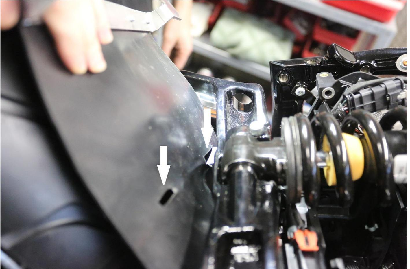
Push the cuttings of the splash guard over the clip of the inner fender.
