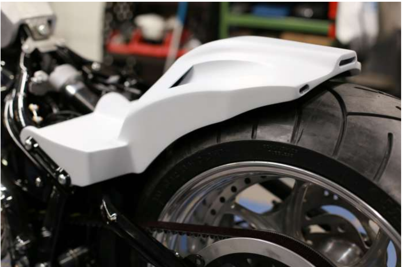
Drill borings for lighting and blinkers wires and for seat mounting.
