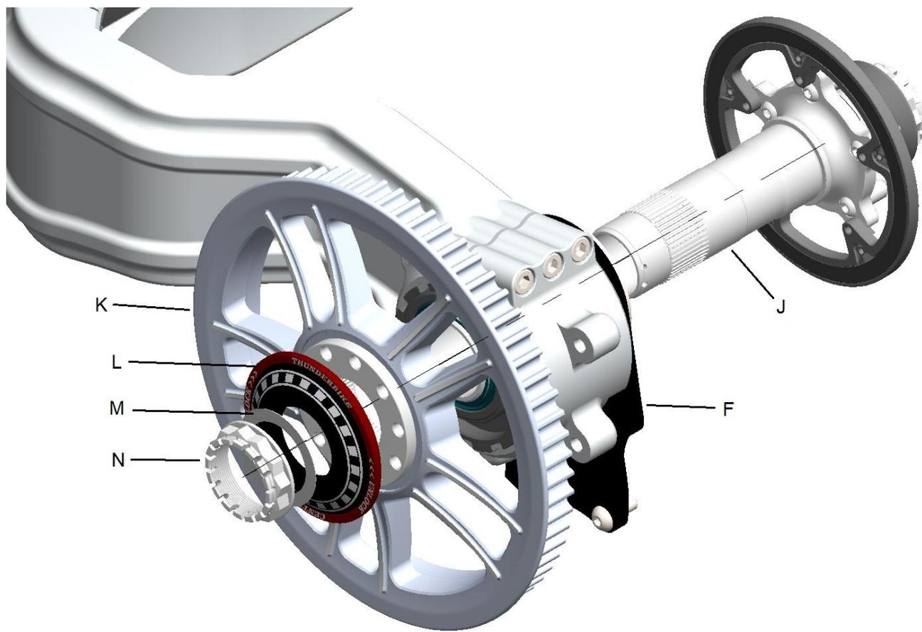
Insert the rear wheel axle (J) from the right side into the excentric. Mount the rear pulley (K), the pulley cover (L), the washer (M) and at least the axle nut (N).
