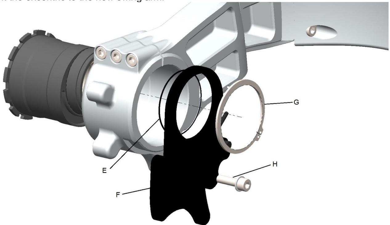
Therefore loosen the three clamping screws and insert the excentric from the left side into the swing arm. Now mount the seal (E) to the excentric first, then the brake caliper bracket (F) and save all with the retaining ring (G). Tighten the bolt (H) by hand.
