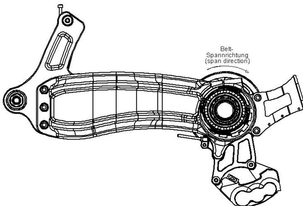
Tighten the three clamping screws with 30Nm torque each now.
