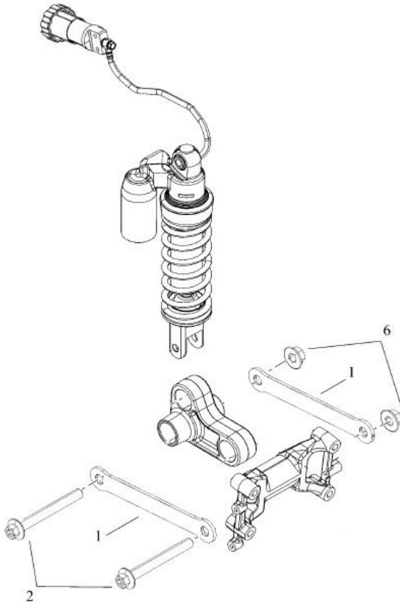
Install the new TB linkage on OEM position using the OEM screws. Tighten the nuts according to the manufacturer's instructions.
