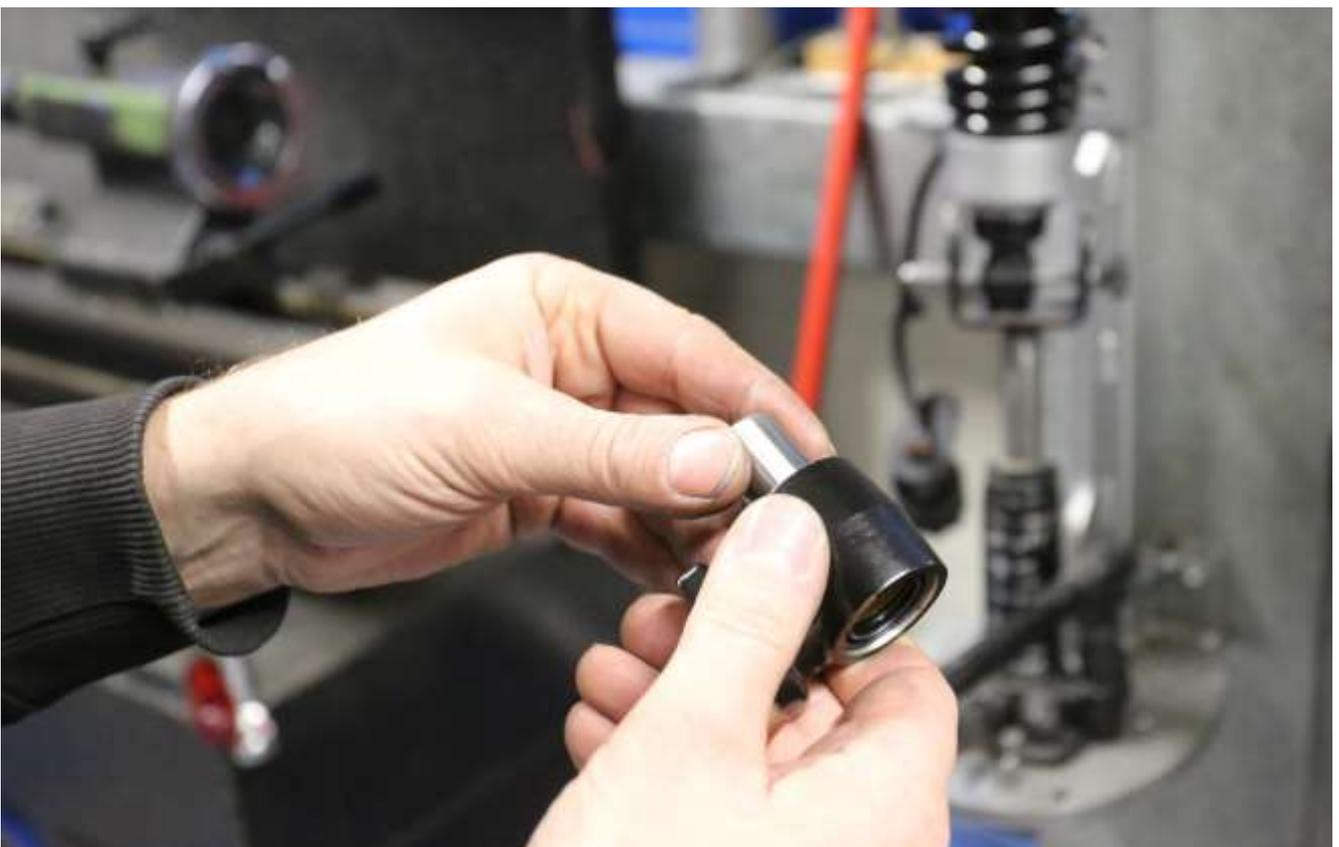
**For Stage 1: Screw the new head onto the piston rod until it blocks. Secure the new head with the counter nut.**
