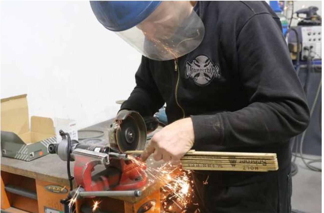
**For 30mm lowering (Stage 2) you have to chop the piston rod by 10mm.
