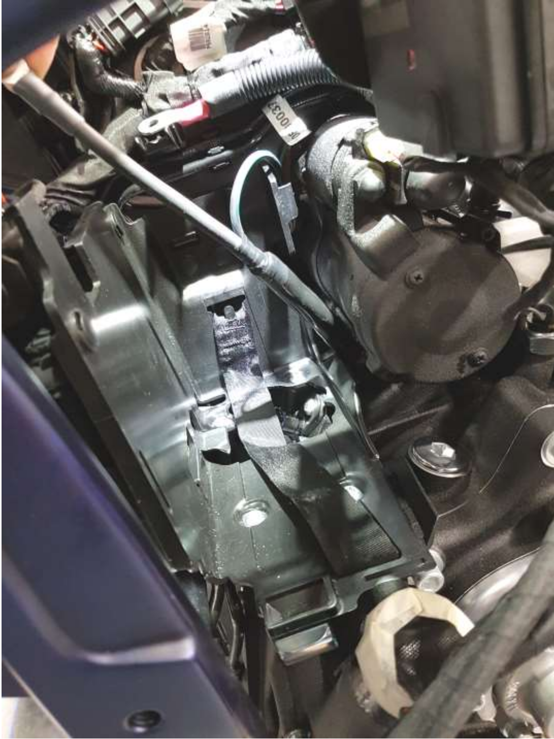
Mount the ground cable with the included spacer to the starter and relocate it between starter and battery box.
