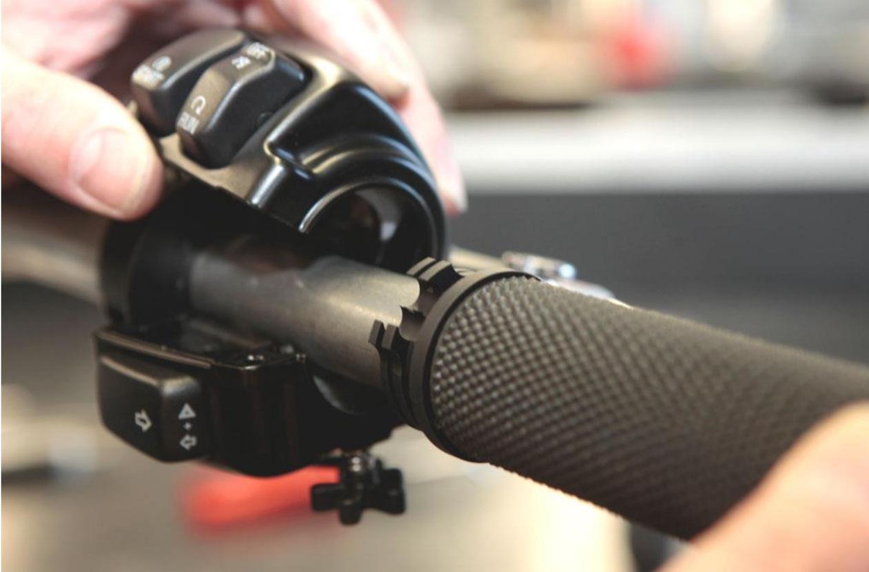
Screw together both parts of the clamp.
