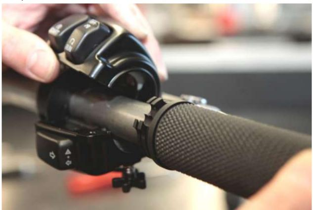
Screw together both parts of the clamp.
