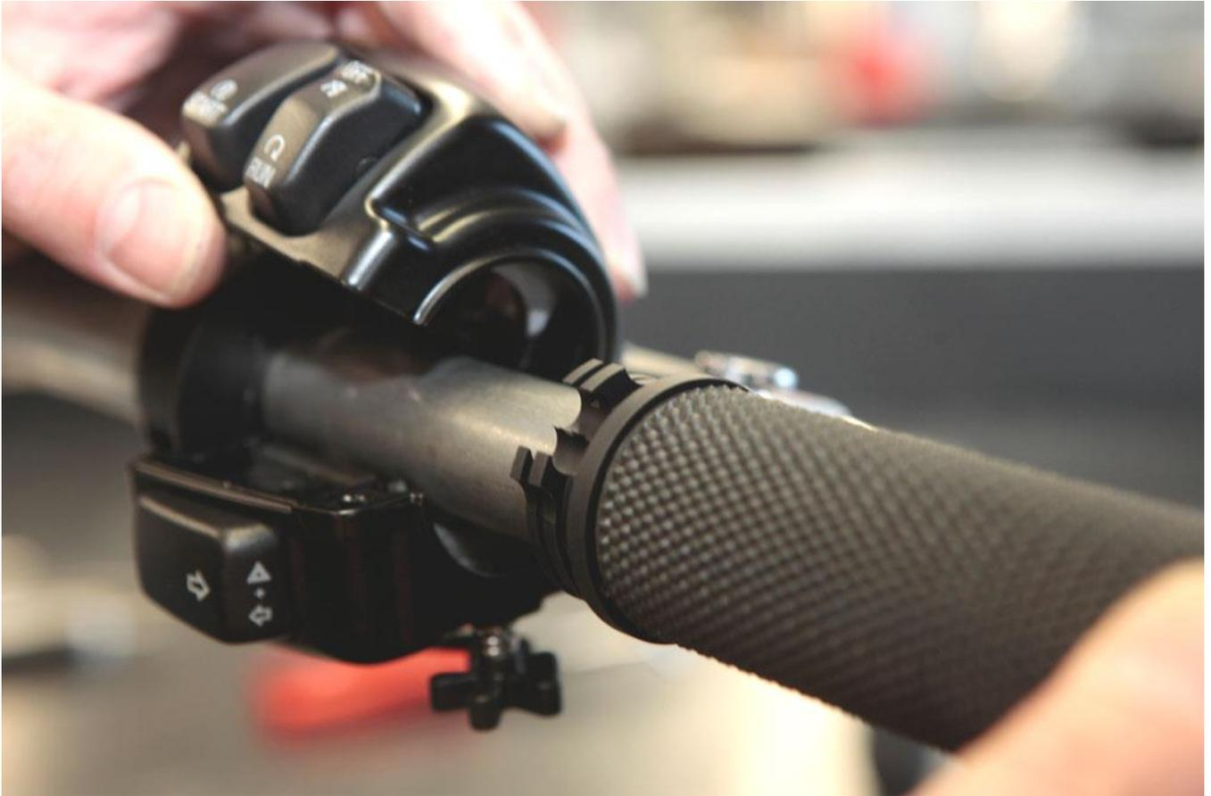
Screw together both parts of the clamp.
