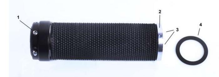
Remove the ring (2) on outer side of the grip and install the grip with the two small screws (3) to the gearing.
