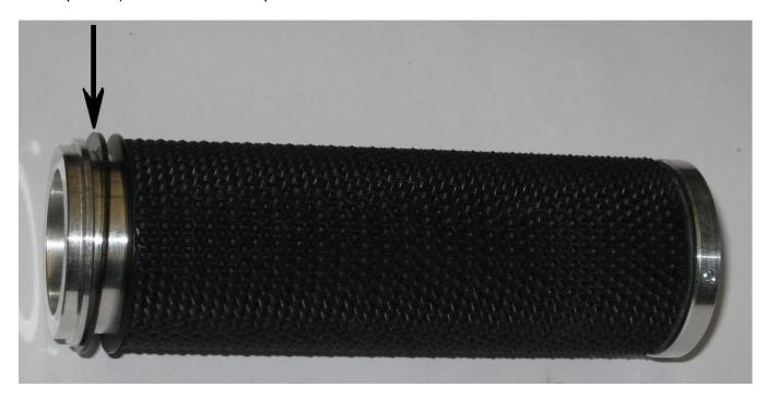
Screw together both parts of the clamp.
