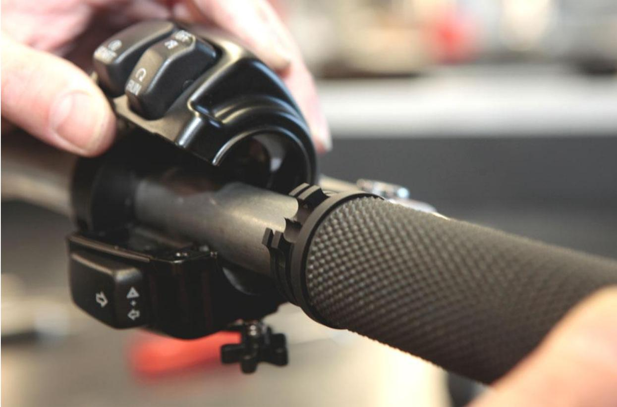
Screw together both parts of the clamp.
