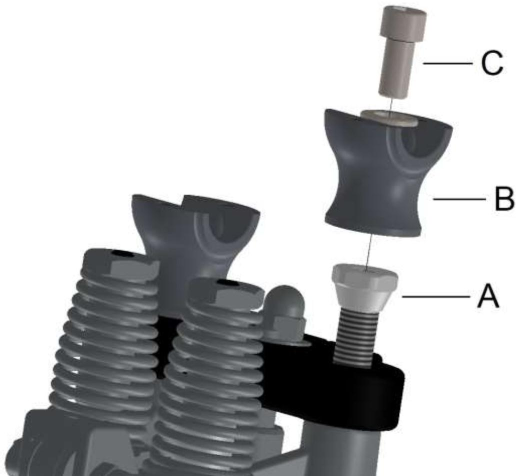
Mount the included adapter (A) to your upper triple tree and tighten it with 81-88 Nm (60-65 ft-lbs) torque.
