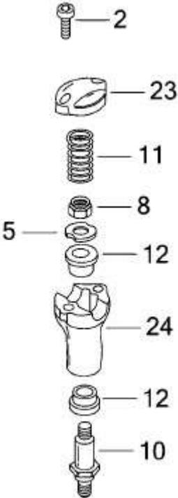
Loosen the clamping screws (2) and remove the upper parts of the OEM risers (23).
