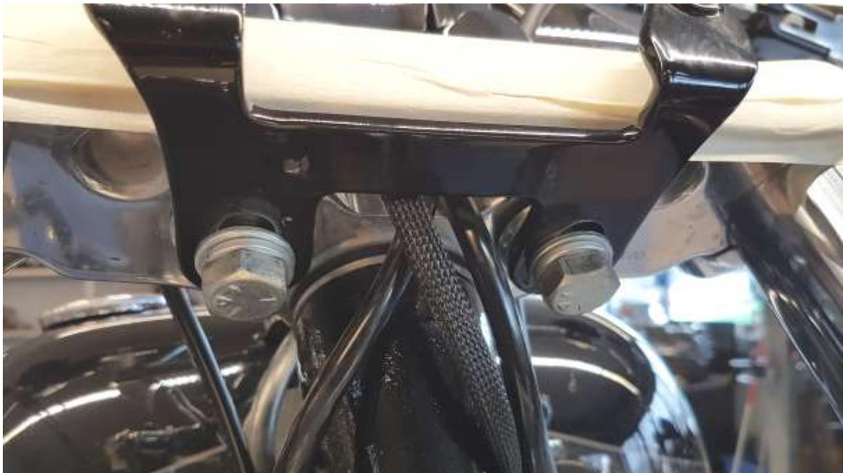
Mount the headlamp cap to the bracket using the included Allen head screws.
