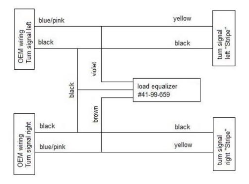
Isolate all the wiring connections you make thoroughly! If it is possible use heat shrink tubing. Make sure that your wiring won't be cut or crimped in use by other items.
