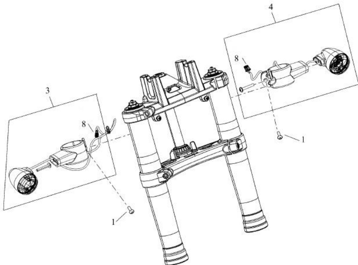
Mount the new TB turn signals onto the fork pipes.
