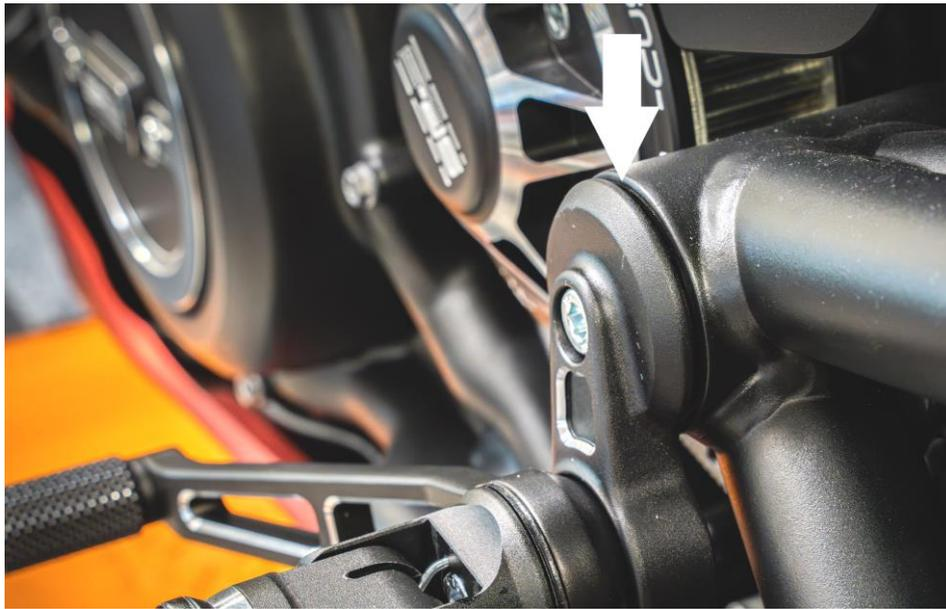
Mount the included shifter rod to the shifting linkage using the Lens flange screw M6\*25, the washer 6\*15 and the acorn nut M6.
