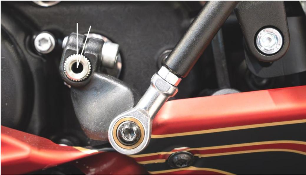
Mount the shifter rod to the bracket using the oem screw.
