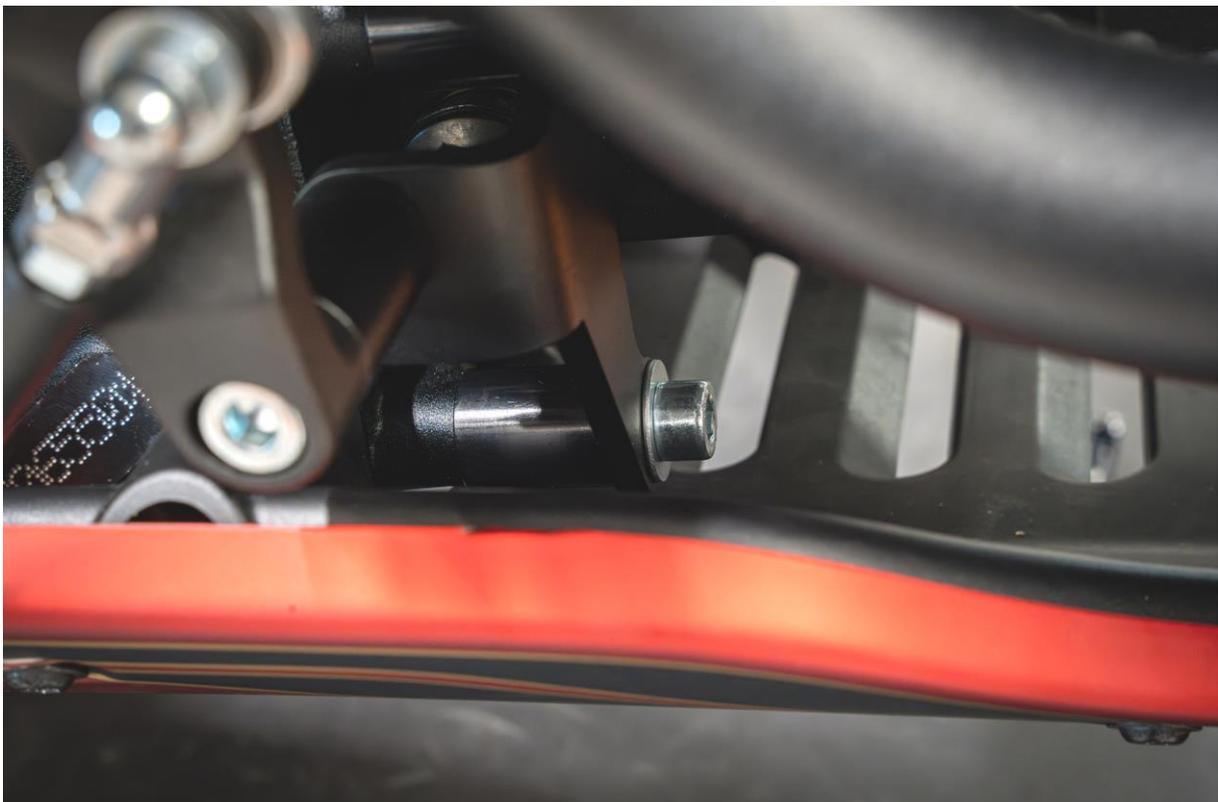
Install the left TB forward control assembly using the included Allen head screws M8\*55 and M8\*30 and tighten the screws with 25 Nm (18,44 ft-lbs) torque.
