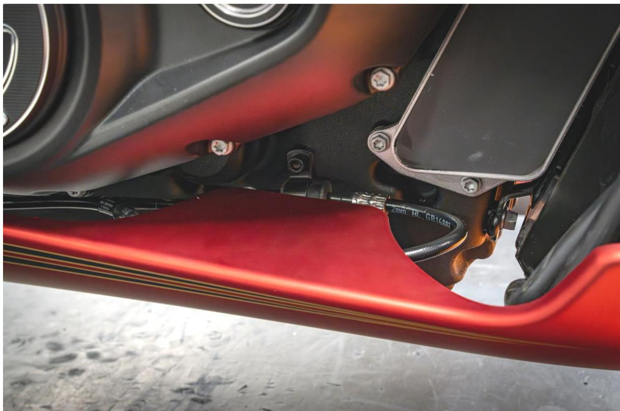
Fill up the brake master cylinder with brake fluid (DOT 4) and bleed the rear brake system.
