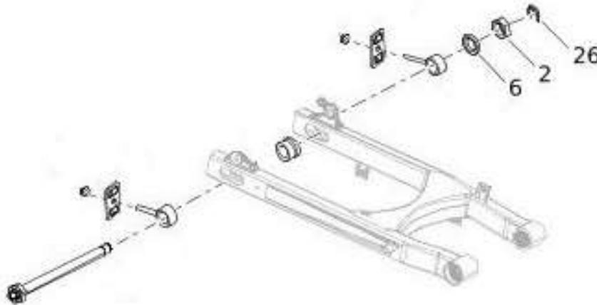
Install the new TB license bracket instead of the washer and tighten the rear axle nut with 140Nm (103,26 ft lbs) torque.
