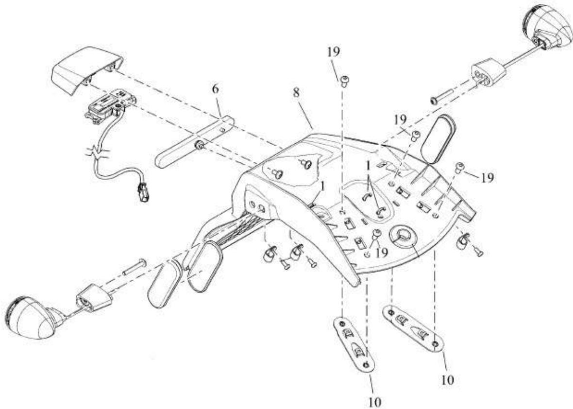
Loosen the four Bolts (19) and remove the brackets (10).
