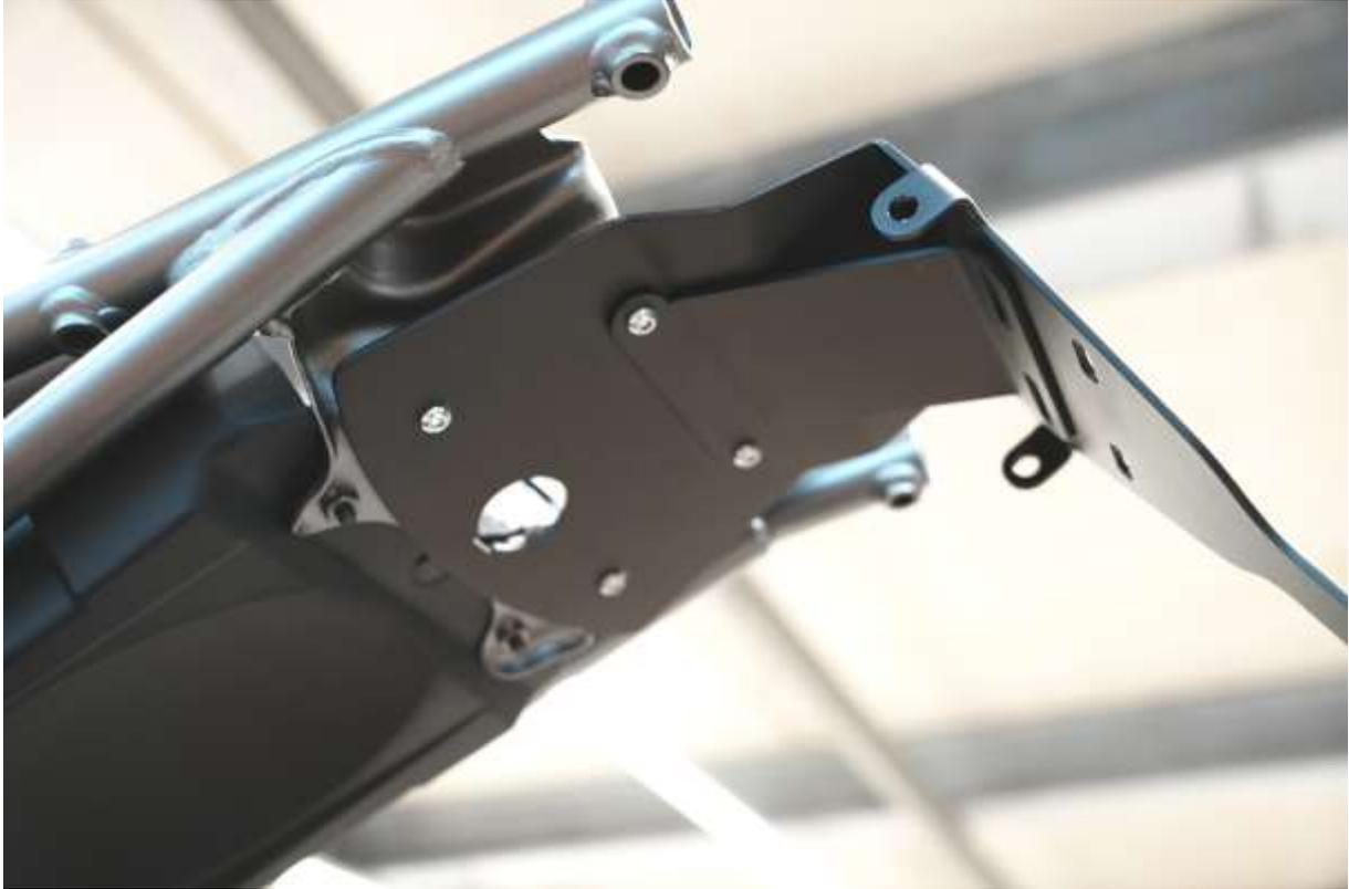
Install the new license plate lightning using the included leans head screws M3\*8 and connect it to the bike.
