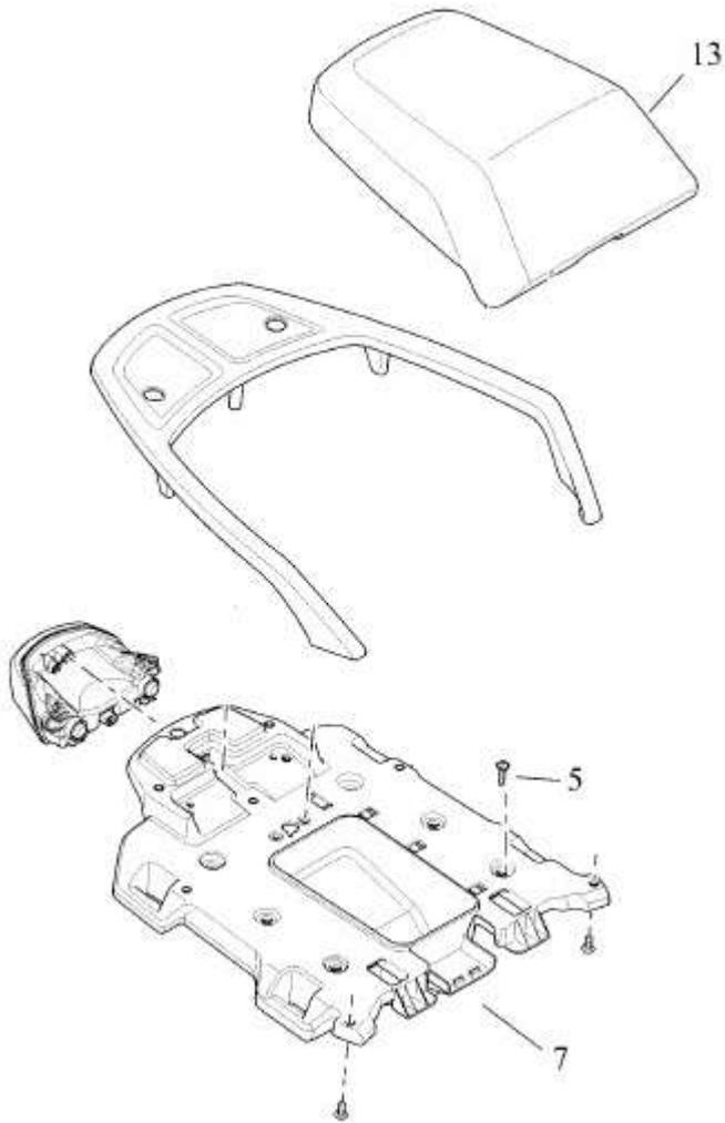
Loosen the four bolts (5) and remove the rear seat plate (7) including the rear light.
