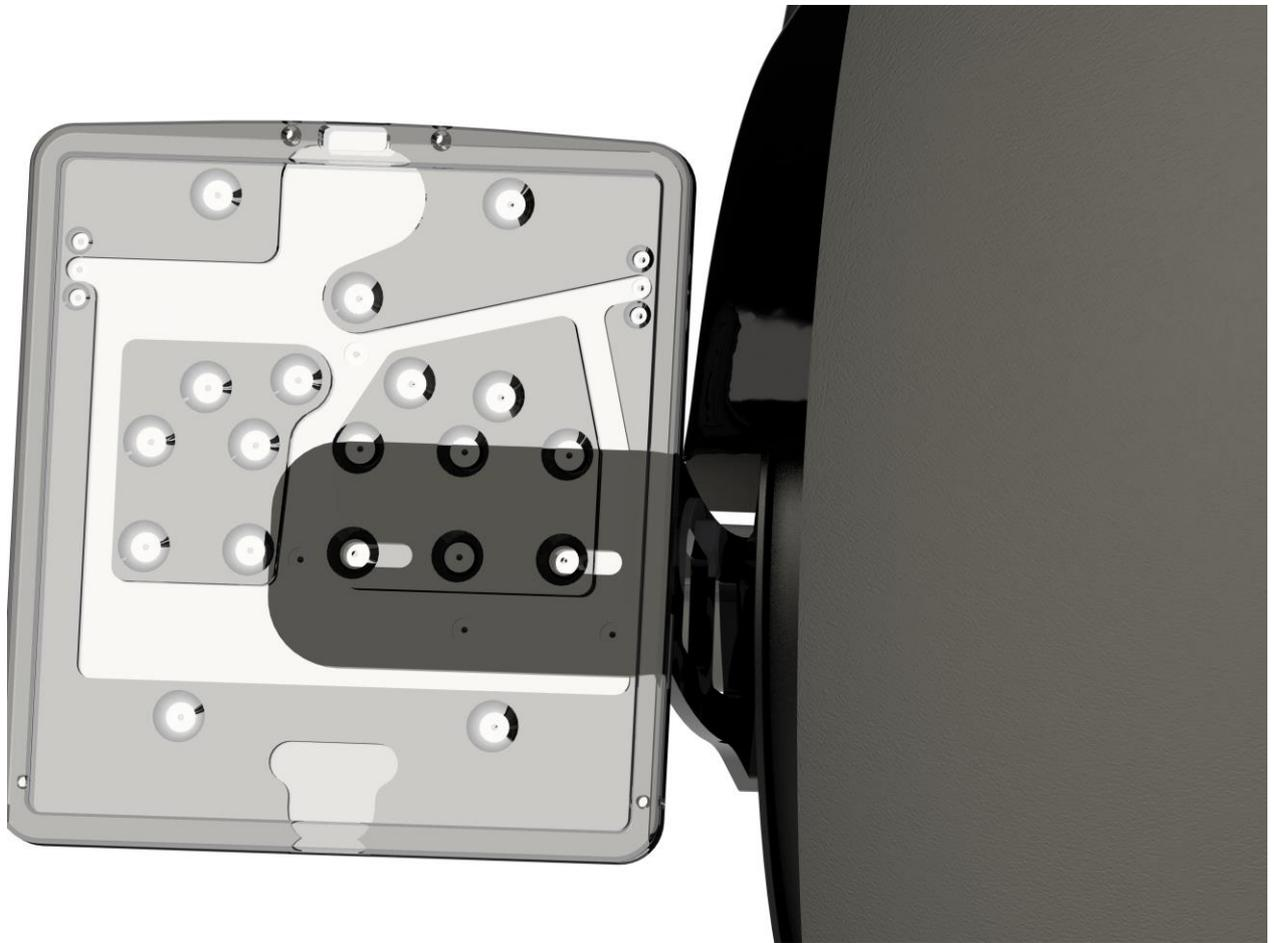
Mount the license plate lightening and connect it to the wiring, make sure the cable doesn't get contact to the wheel! Fix the cable with the straps.
