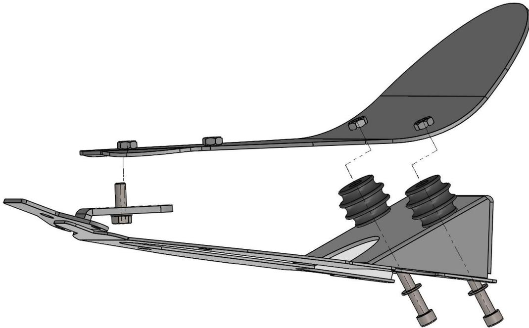
Mount the frame plate with the front seat bracket to the frame.
