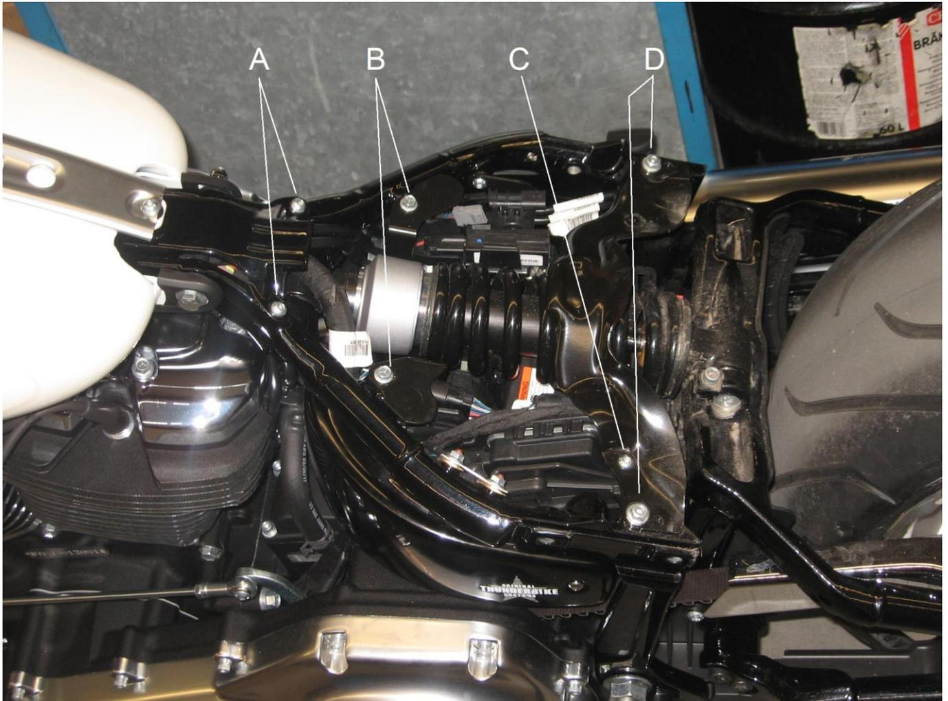
Remove the screws (A,B,C,D) and remove the front seat bracket and the rear cross brace.
