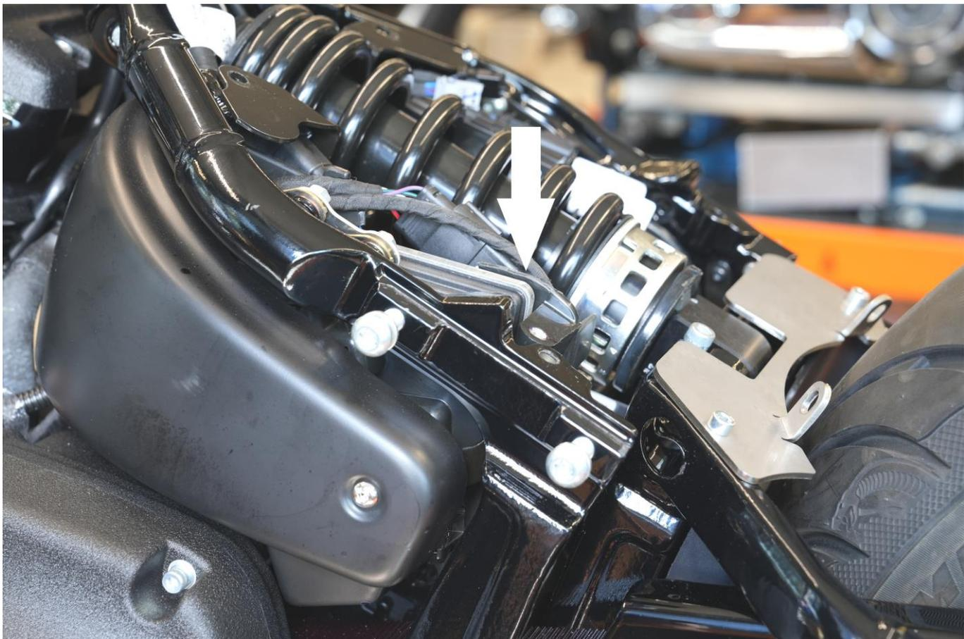
Install the spring imitates (3) and seat bracket (4) to the frame cover.
